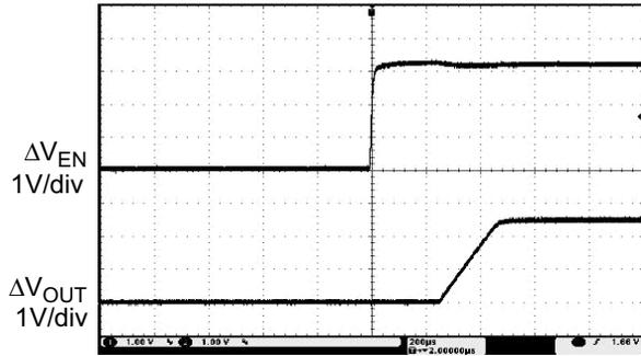
Figure 20. Enable Input Response
